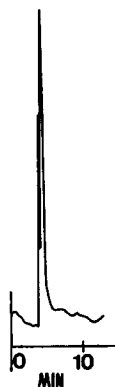
Fig. 4. Electropherogram of a sample of protamine. Electrophoretic conditions: 5 mg/ml F-108 modified column, 43 cm (31 cm effective length) \times 50 \mu m I.D.; 0.01 M phosphate-borate, pH 5.5; voltage: 15 kV; wavelength: 200 nm.
